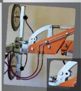
settings, adjusted by means of two holes for the locking bolt. The lifting head can therefore be adjusted to tilt more towards the ceiling or floor.
